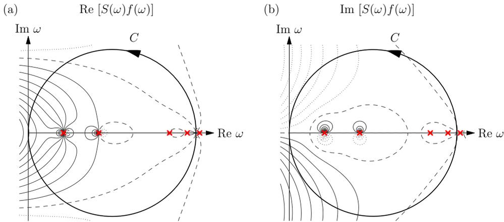
FIG. 1. (Color online) Schematic representation of the integration contour  $C$  used to evaluate beta-decay rates. Only the poles of the strength function below the endpoint energy  $\omega_{\max}$  contribute to the decay rate.
